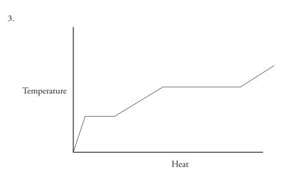
The diagram above shows how the temperature of a certain covalent substance changes as heat is added to it.
